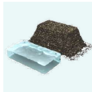
Traditional aggregate 30% Void ratio
